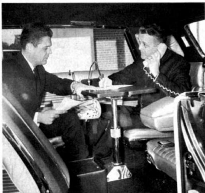
The Executive accommodates a separate radio telephone for voice transmission. The front passenger seat swivels 180 degrees to the rear to allow comfortable meetings over the steady desk. Center armrest contains most of the gear.
